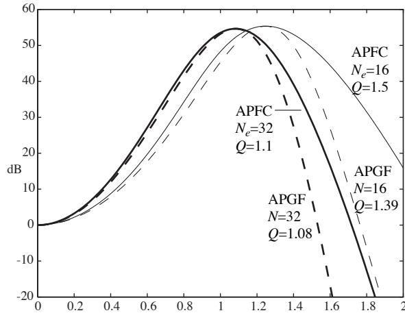
Figure 3: Comparison of APGF and APFC transfer functions. The frequency axis is labeled in units of the tap natural frequency, and parameters are noted in term of pole  $Q$ . The APFC needs a large number of stages per factor of  $e$  frequency change ( $N_e$ ) to approximate the APGF shape.
