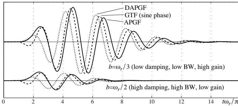
Figure 2: Impulse responses of the APGF, DAPGF, and sine-phase GTF from Figure 1. Note that the GTF's zero crossings are equally spaced in time, while those of the APGF and DAPGF are stretched out in the early cycles.
