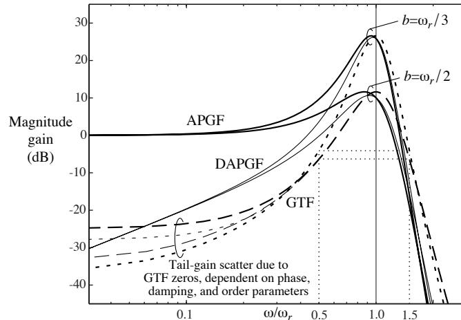
Figure 1: Comparison of GTF, APGF, and DAPGF transfer functions ( $N = 6$ ) for two different values of the real part of the pole location. Dotted lines show the symmetry of the GTF at  $f = 1 \pm 0.5$ . Each GTF is shown with two phases (0 and  $\pi/2$ , heavy and light dashed lines, respectively). Notice that the ordering of gain near the peak is not maintained in the tail. The variation in the GTF tail is not accounted for by the usual phase-independent symmetric GTF approximation.
