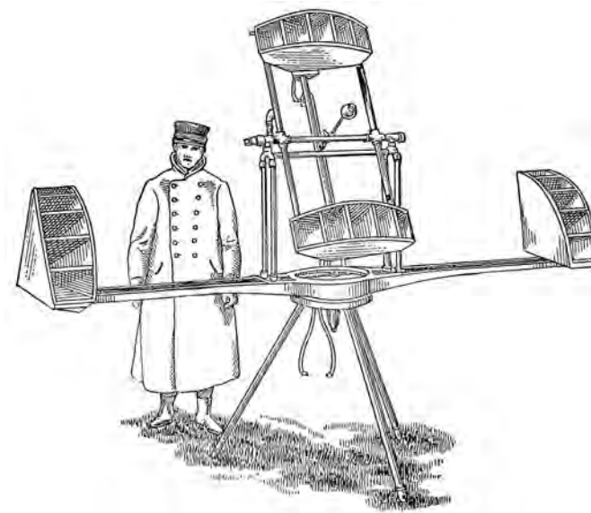
Figure 22.2: A World War I era acoustic goniometer for locating “invisible aeroplanes” (Ferry, 1921). Operators rotate pairs of pickup horns about vertical and horizontal axes, until a sound seems to be straight ahead. The device is clearly designed to exaggerate an interaural time difference cue.
